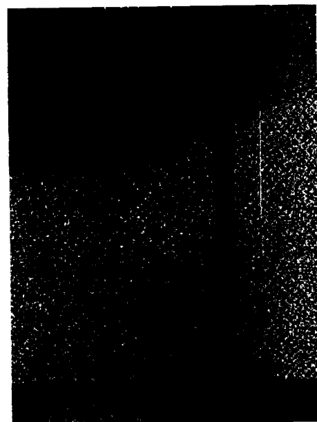
Fig. 3. Nickel map of EDAX/SEM photograph ( 5000\times ) of the Ni-coated alloy particle of Fig. 1.
